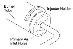
Figure 44 - Injector Holder On Outlet Burner Tube
